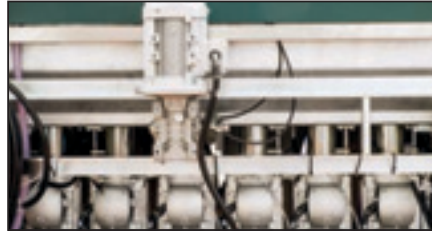
Spindles are equipped with independent motors and encapsulated, waterproof bearings.
