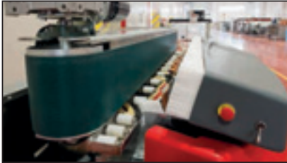
Adjustable belt speed is achieved using speed settings and inverter for functionality.
