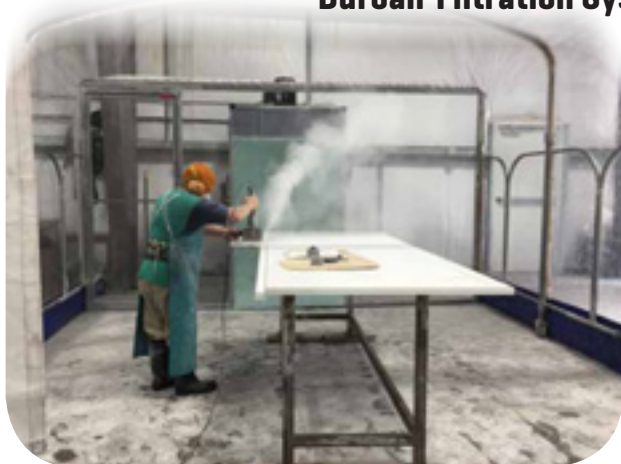
Retractable dust enclosure closes to 20% of the extended length allowing for maximum use of shop space.
