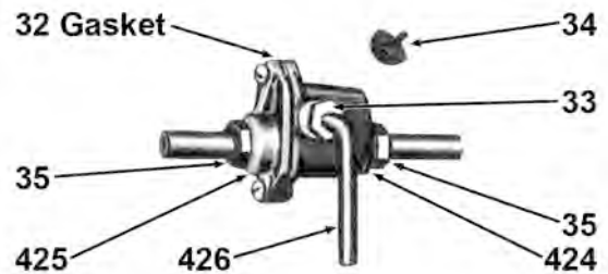
Blast Control Valve
