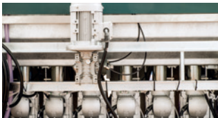
Spindles are equipped with independent motors and encapsulated, waterproof bearings.
