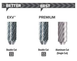
The **Double Cut** is the most popular bur for ferrous materials. The flutes are precision ground in both left and right directions, offering aggressive stock removal and a smooth finish.
